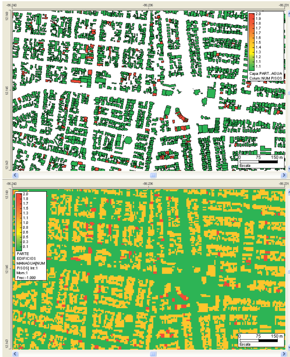
Figure 56 Rasterization result of a shapefile. Left original shape and right generated raster
